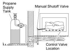
Figure 16 - Checking Gas Joints
